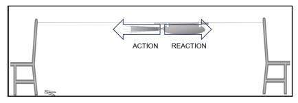
Q3. The air would rush out of the balloon due to the elastic energy in the balloon. The model balloon rocket would propel very fast to the right as soon as the air gushes out. The balloon would travel fast until the air is gone, then it would slow and stop because of the friction of the straw on the string.
